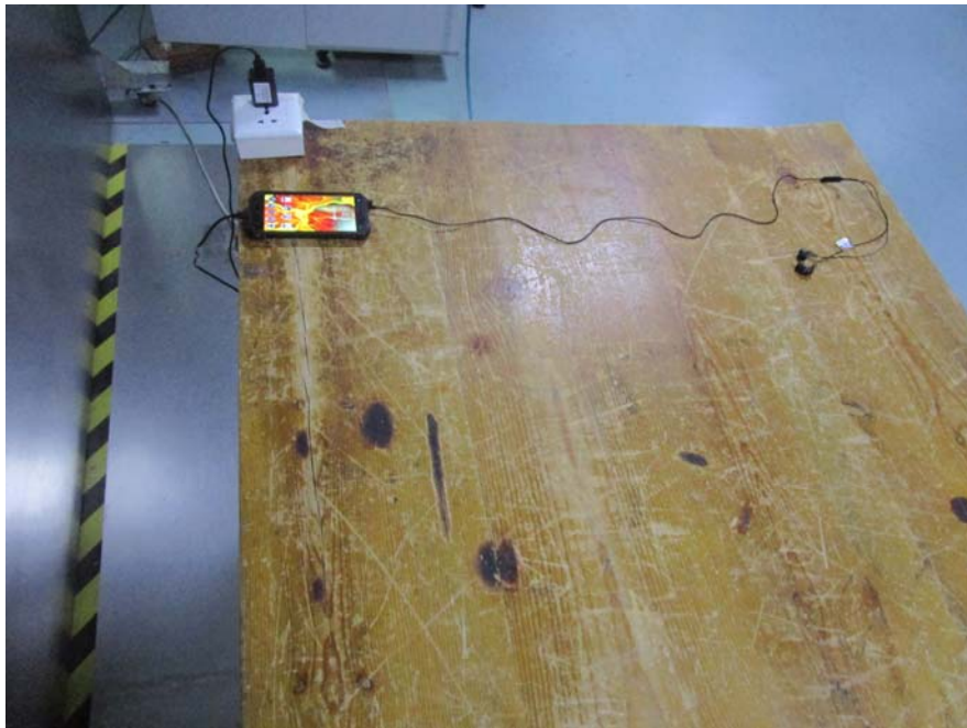
Conducted Emissions – Side View
