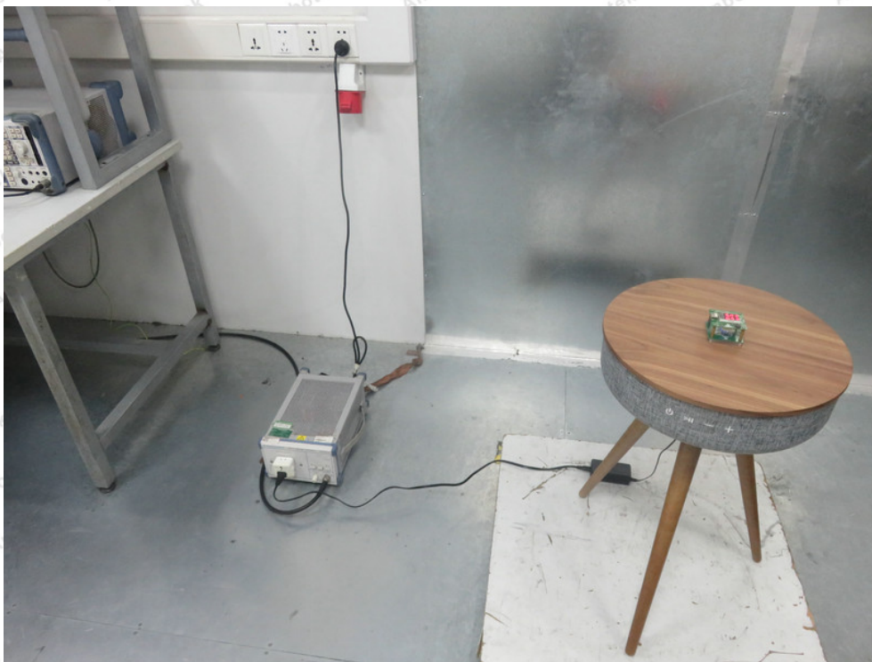
Photo of Conducted Emission Measurement
