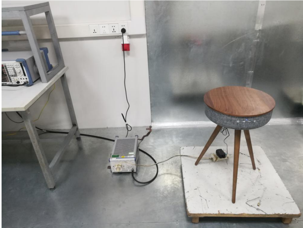
Photo of Conducted Emission Measurement
