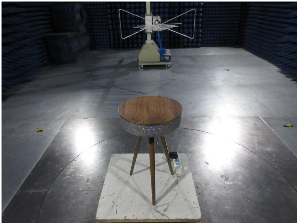
Photo of Radiation Emission Test
