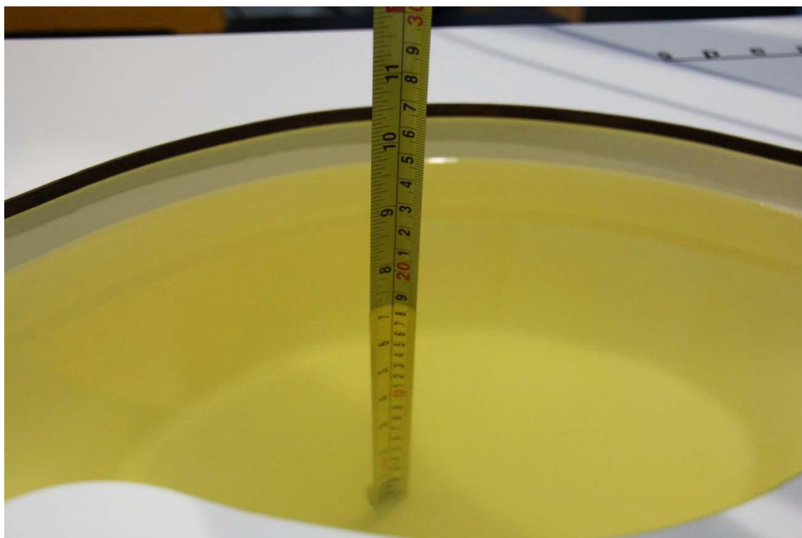
Picture 7-1: Liquid depth in the Flat Phantom(2450MHz)
