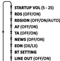
Select any one of the above settings and rotate the knob to setup.
