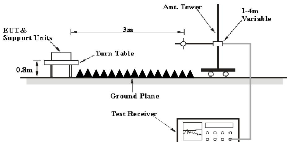
The radiated emission tests were performed in the 3 meters chamber test site for the range 30MHz to 1GHz and the 3 meters chamber test site for above 1GHz, using the setup accordance with the ANSI C63.4-2014. The specification used was the FCC Part 15.109 Class B limits.
