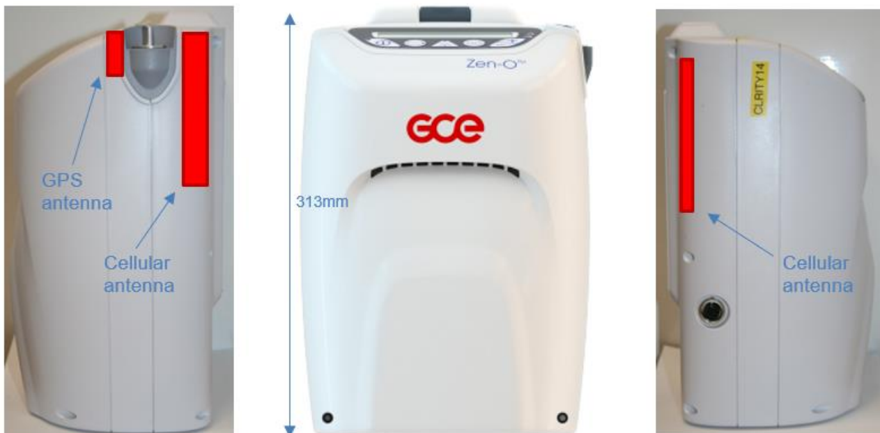
The location of the antenna
