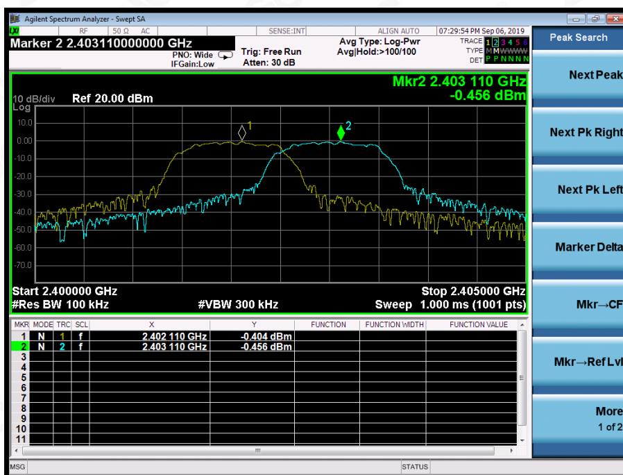
TEST PLOT FOR FREQUENCY SEPARATION
