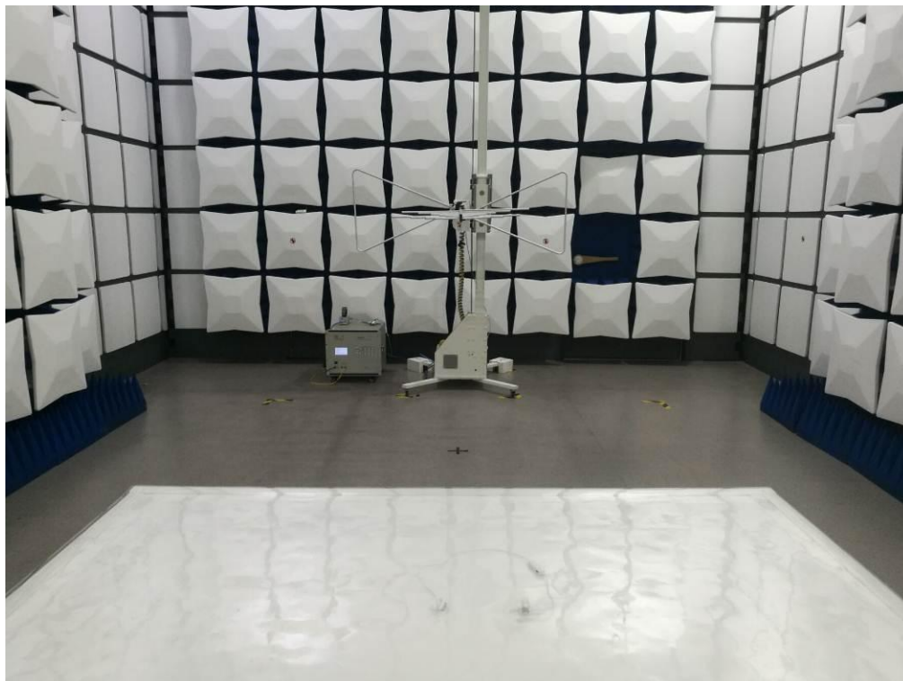
FCC RADIATED EMISSION TEST SETUP
