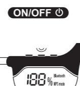
**Power ON:** Press and hold the Power Button for 2 seconds until the LCD Screen display Battery Level and Bluetooth mode with "power on" prompt sound.
