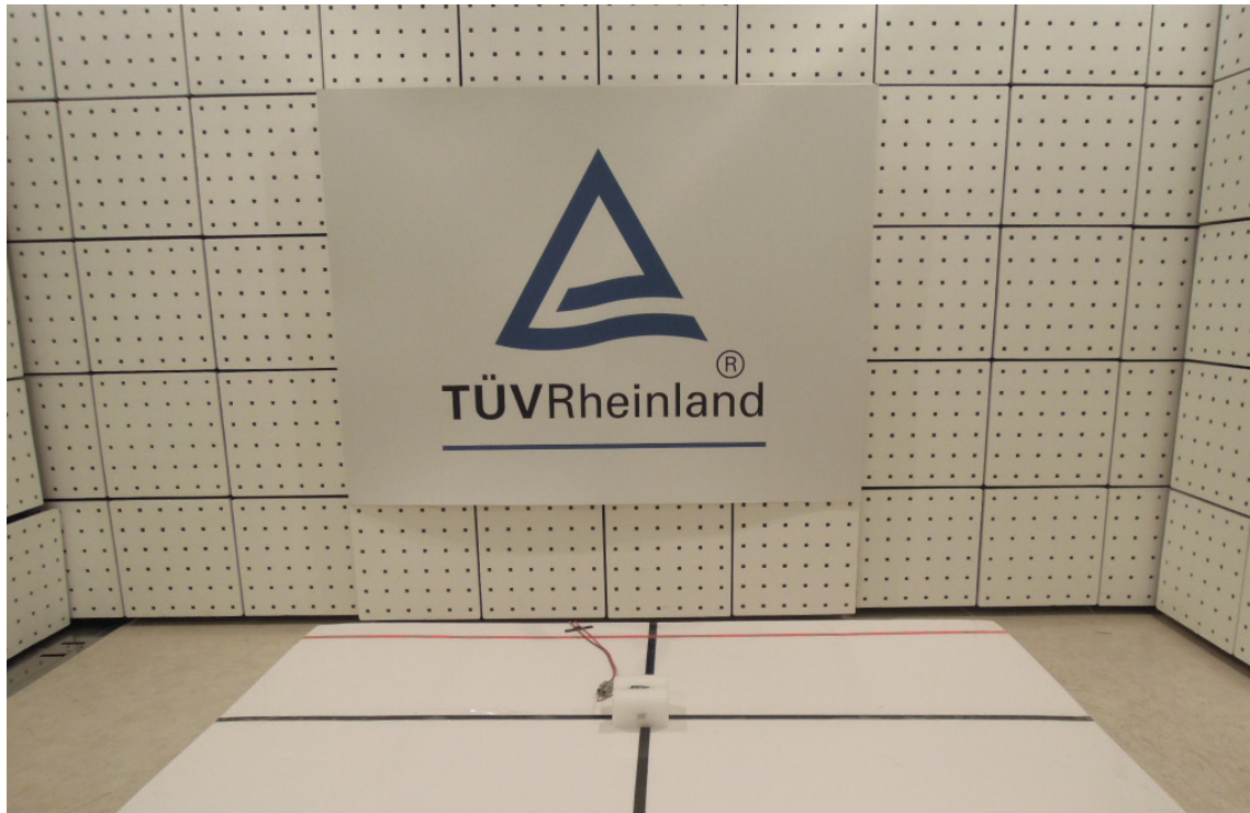
Photograph 1: Set-up for Spurious Emissions (Front View 1)
