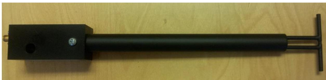
Figure 1 – MVG COMOSAR Validation Dipole
