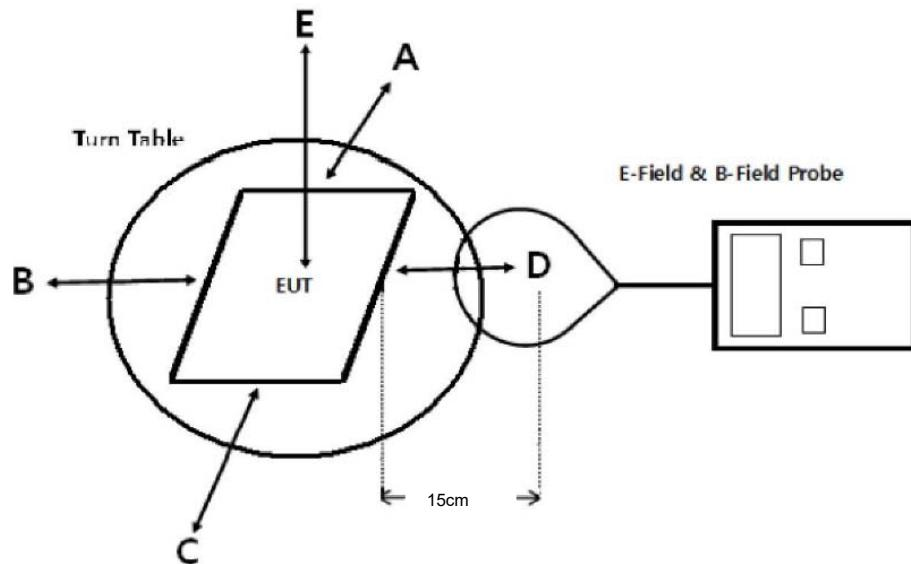
Note: The aggregate H-field strengths at 15 cm surrounding the device and 20 cm above the top surface.
