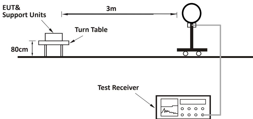
**For Radiated emission 30MHz to 1GHz:**
