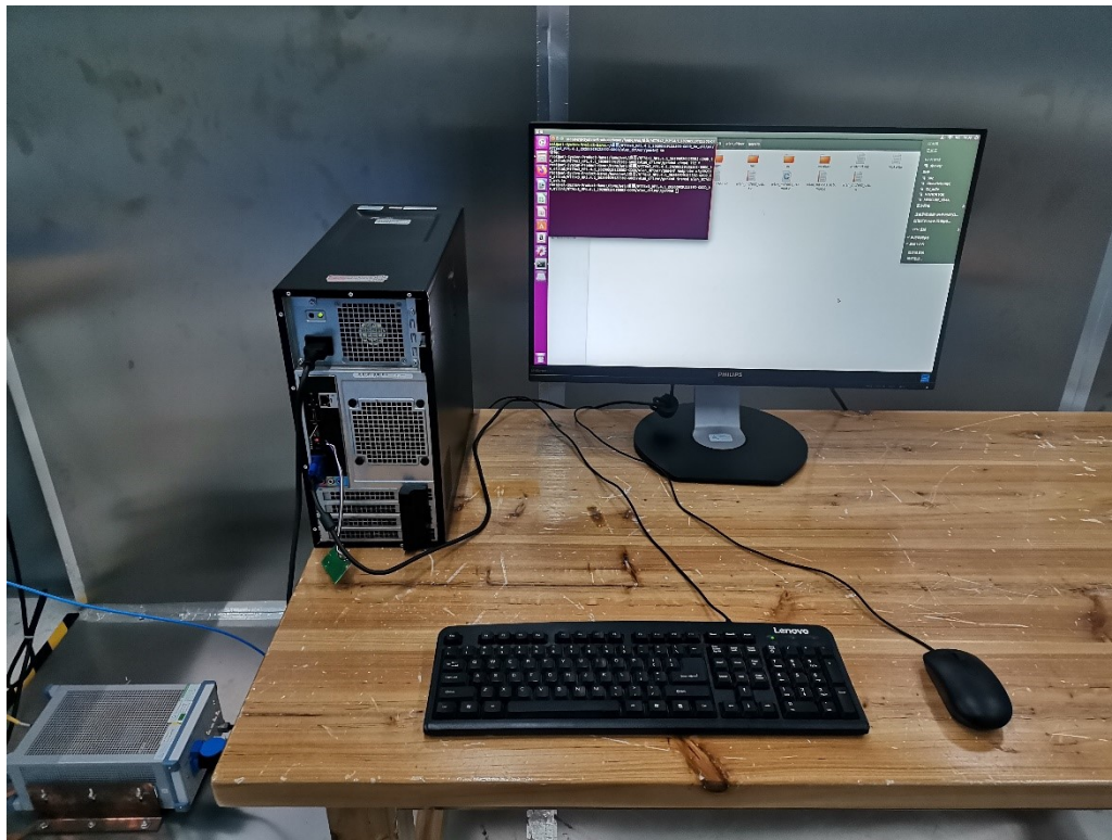
Photograph 3: Set-up photo for AC Conducted Emissions
