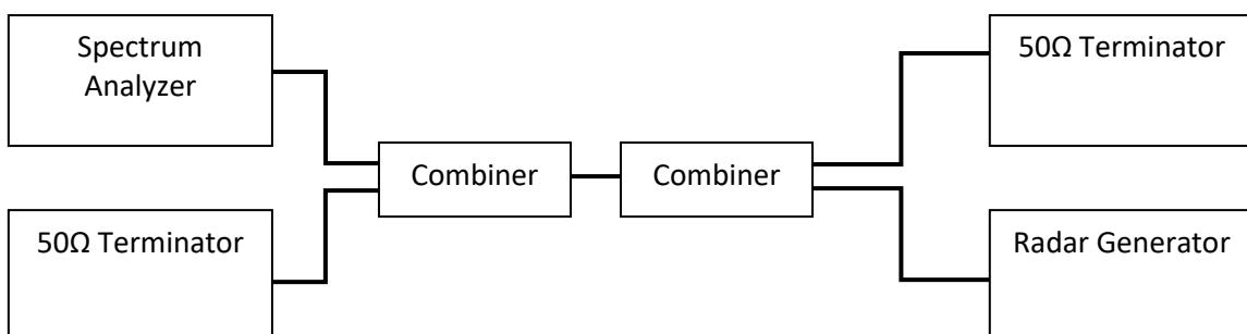
**TEST REPORT****3.8 Radar Waveform Calibration Procedure**
