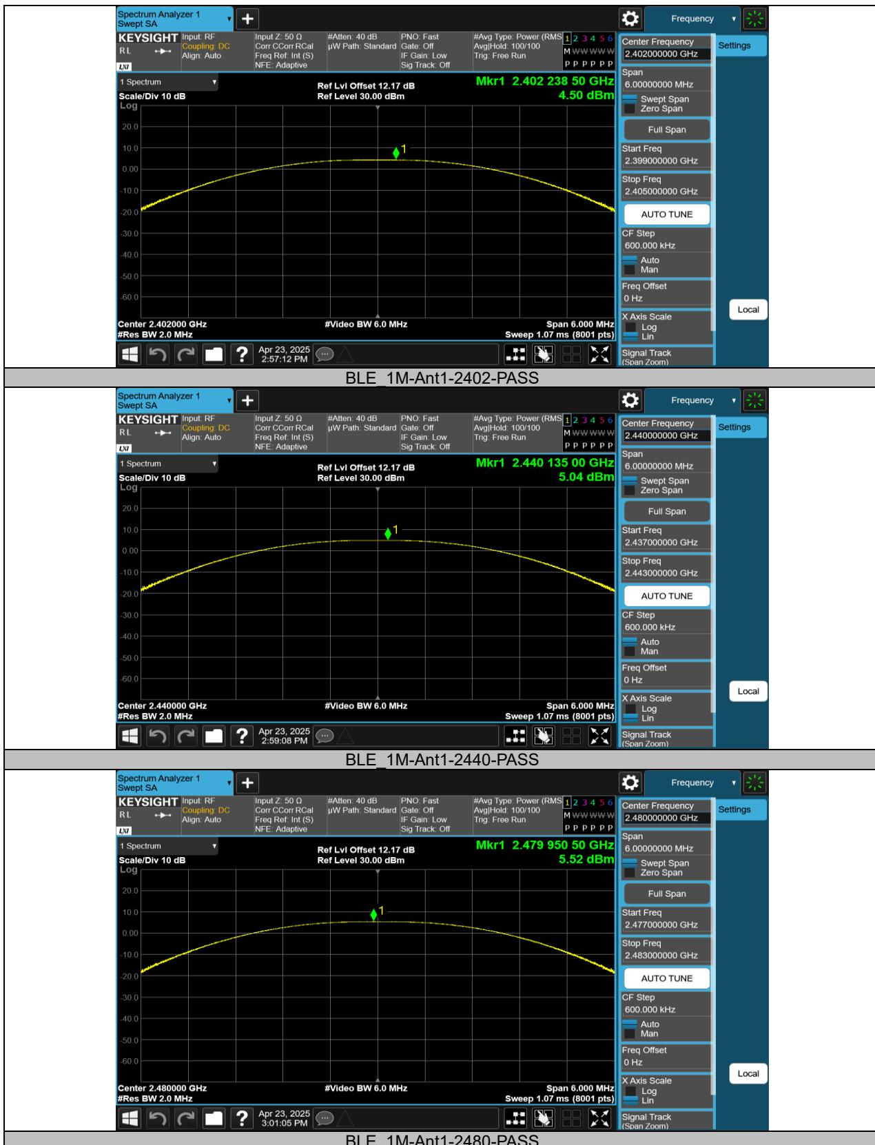
**TEST REPORT****Maximum power spectral density****Test Result**
