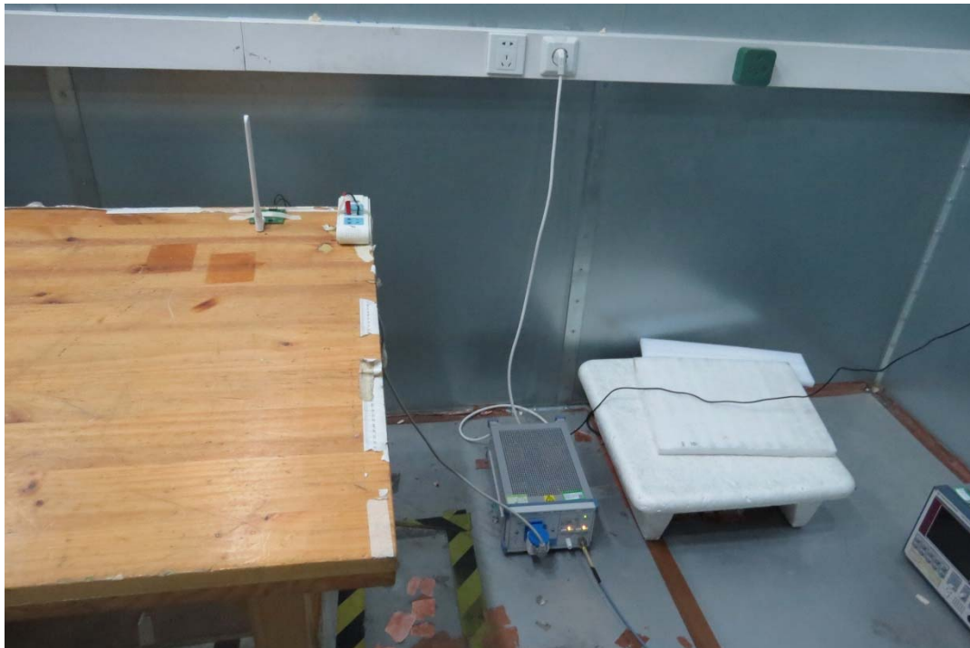
Picture 3 Conducted Emission Test Setup
