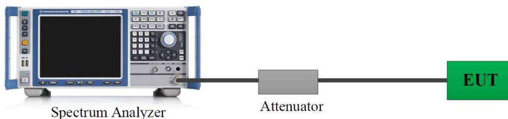
A short RF cable with low cable loss connected to the EUT antenna port. The insert loss of this RF cable/attenuator was offset into the setting of test equipment.
