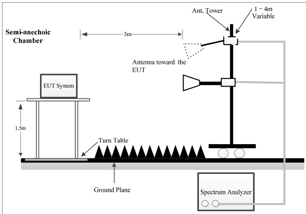
The radiated emissions were performed in the 3 meters distance, using the setup accordance with the ANSI C63.10-2020. The specification used was the FCC 15.209, and FCC 15.247, RSS-247, RSS-Gen limits.
