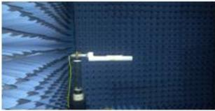
[Fig.2] DUT JIG(Quiet Zone 20Cm)
