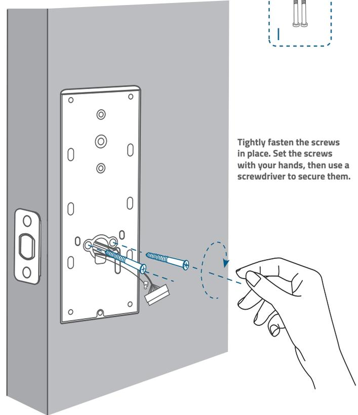
4. (Optional) If the back cover is not fastened tightly to the door, use the additional screw provided.
