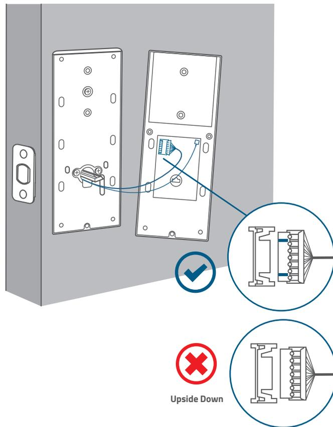
6. Mount the interior assembly. **Make sure both wires are tucked into the cabin on the back of the interior assembly.**
