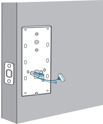
3. Secure the back cover with screws.
