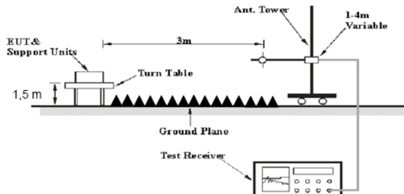
The radiated emission below 1GHz tests were performed in the 3 meters chamber A, above 1GHz tests were performed in the 3 meters chamber test site B, using the setup accordance with the ANSI C63.10-2013. The specification used was the FCC 15.209, FCC 15.247, RSS-247 §5.5, RSS-Gen §8.10 limits.
