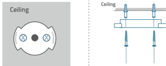
4. Align the grooves with the mounting plate and rotate the eufy Indoor Cam clockwise until it clicks into place.
