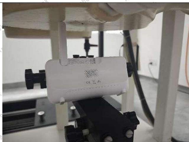
Body Top(0mm) Antenna bends 90 degrees
