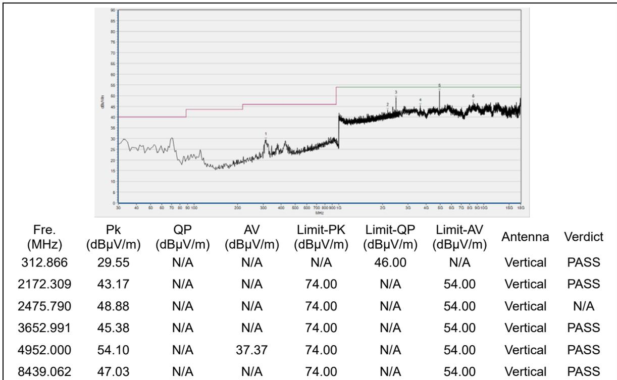
(30MHz to 18GHz, Antenna Vertical, GFSK, channel 20)
