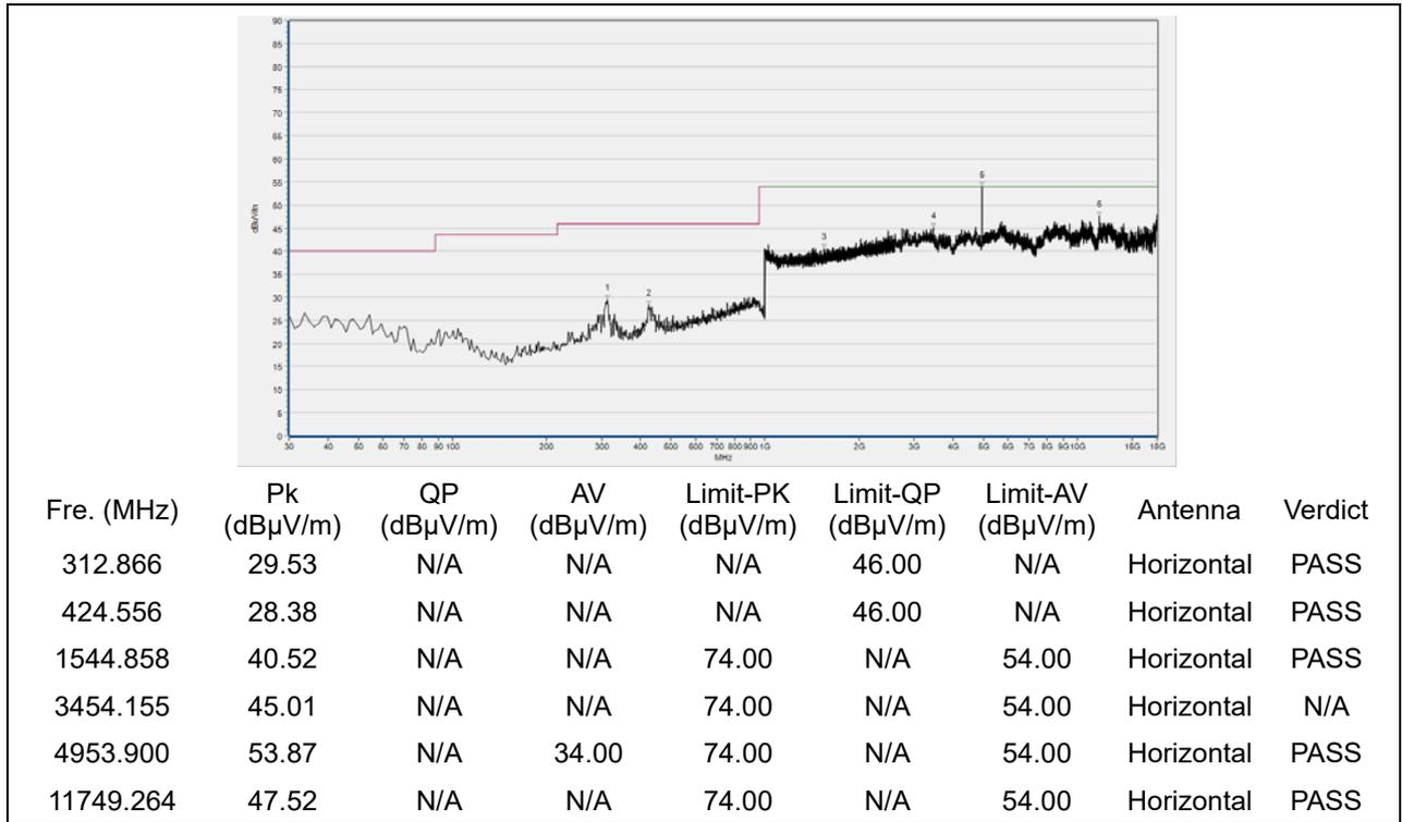
(30MHz to 18GHz, Antenna Horizontal, GFSK, channel 20)
