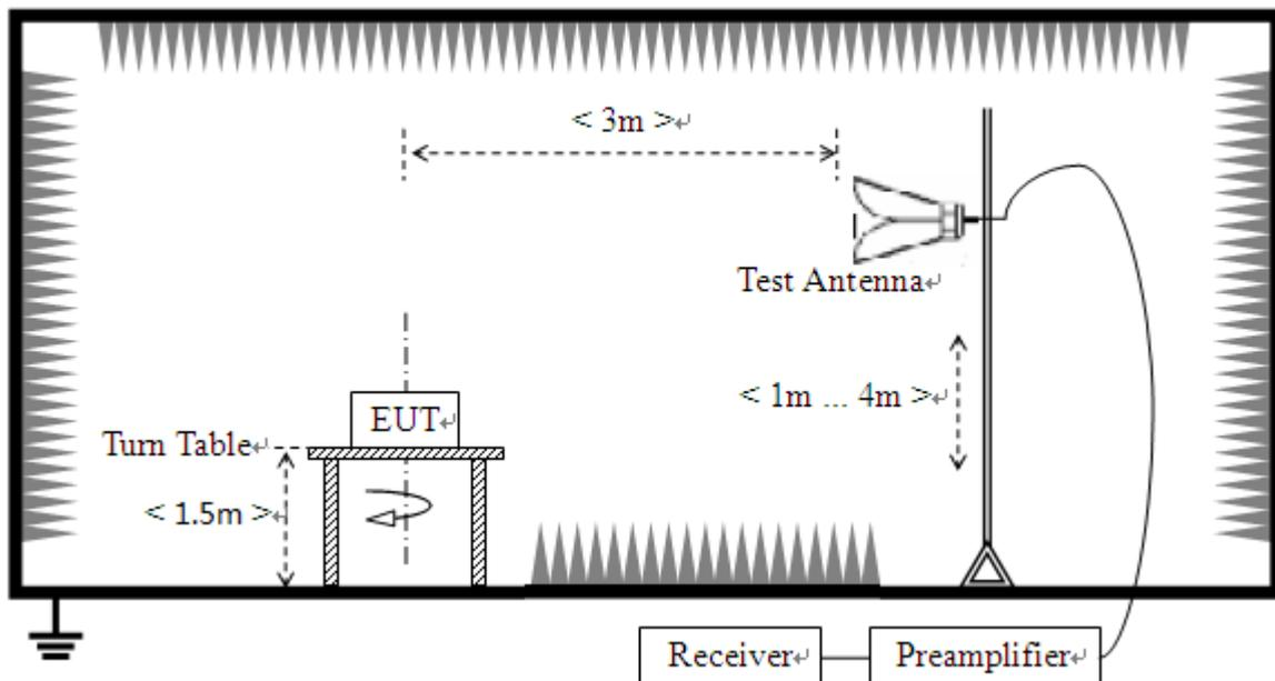
The EUT is located in a 3m Semi-Anechoic Chamber; the antenna factors, cable loss and so on of the site as factors are calculated to correct the reading.
