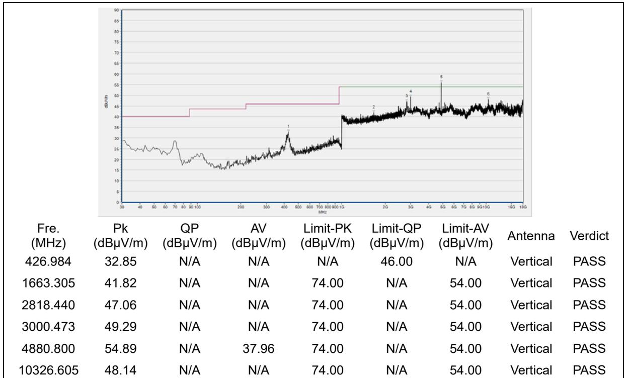
(30MHz to 18GHz, Antenna Vertical, GFSK, channel 10)
