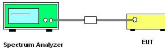
The EUT (Equipment under the test) is coupled to the Spectrum analyzer; the RF load attached to the EUT antenna terminal is 50Ohm; the path loss as the factor is calibrated to correct the reading, all test result in Spectrum analyzer.
