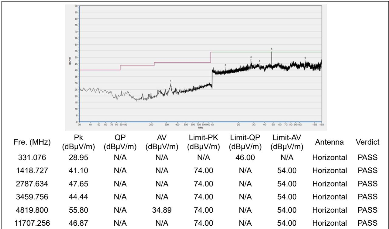
(30MHz to 18GHz, Antenna Horizontal, GFSK, channel 1)
