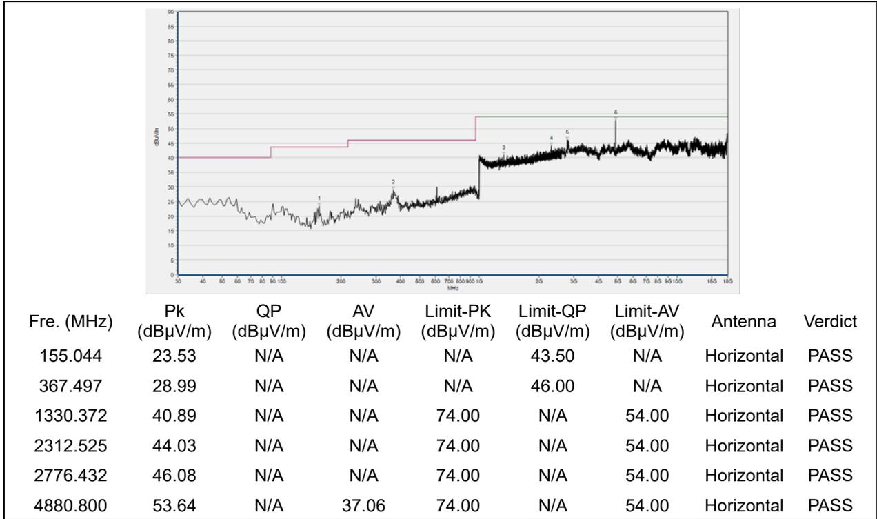
(30MHz to 18GHz, Antenna Horizontal, GFSK, channel 10)
