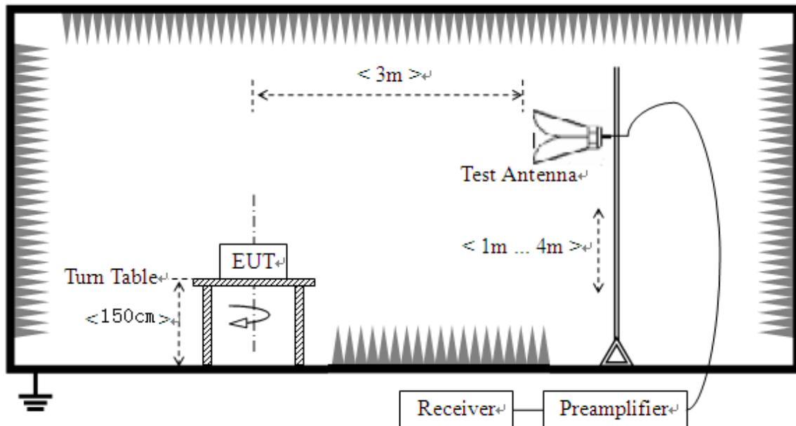
The RF absorbing material used on the reference ground plane and on the turntable have a maximum height (thickness) of 30 cm (12 in) and have a minimum-rated attenuation of 20 dB at all frequencies from 1 GHz to 18 GHz.
