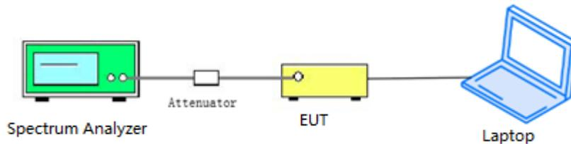
The EUT is coupled to the Spectrum Analyzer; the RF load attached to the EUT antenna terminal is 50Ohm; the path loss as the factor is calibrated to correct the reading.
