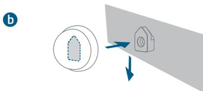
3. Attach eufyCam 2 Pro to the indoor mount and adjust the viewing angle.
