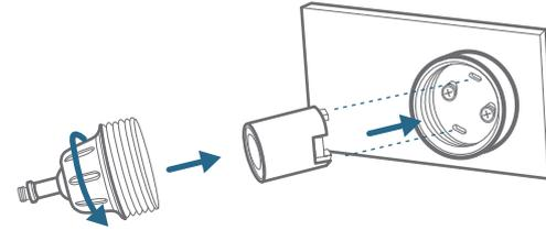
4. Tighten eufyCam 2 Pro to the mounting bracket and adjust the viewing angle by checking the live stream feed in the eufy Security app.
