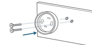
3. Firmly screw the base of the mounting bracket onto the wall. Fasten the ball knob of the bracket to the base of the bracket.
