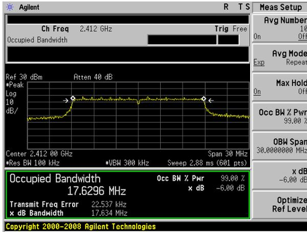
(802.11 N40) 6dB Bandwidth plot on channel 3
