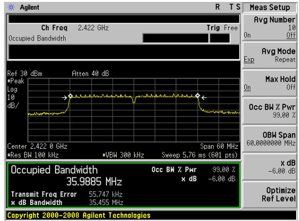
(802.11 N20) 6dB Bandwidth plot on channel 6
