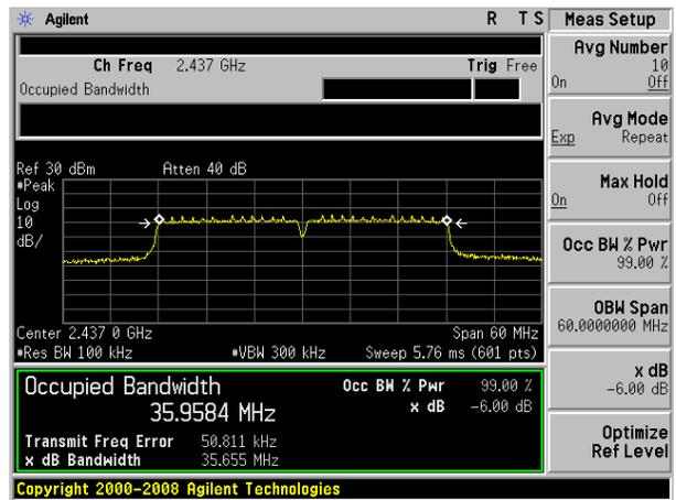
(802.11N20) 6dB Bandwidth plot on channel 11
