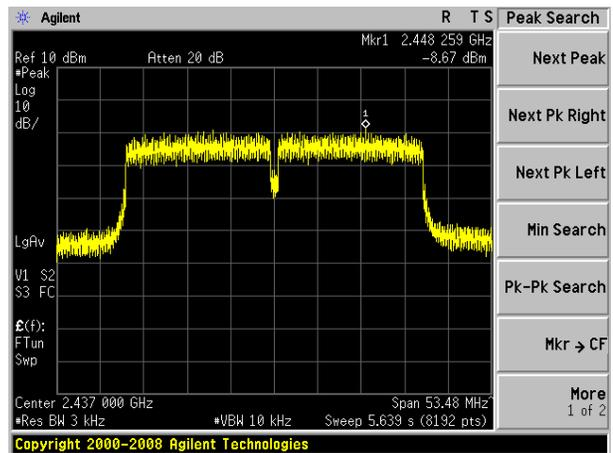
(802.11n20) PSD plot on channel 11
