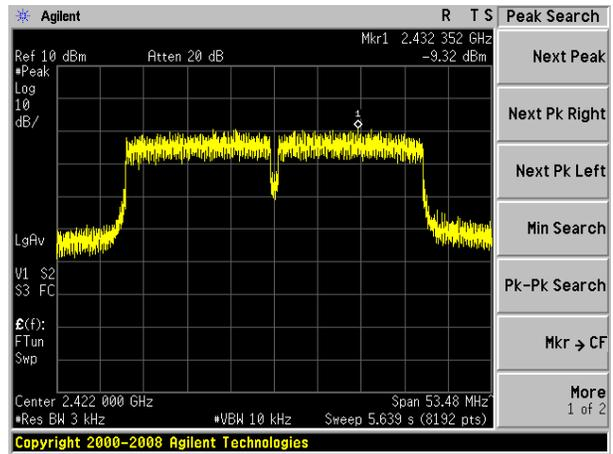
(802.11n20) PSD plot on channel 6
