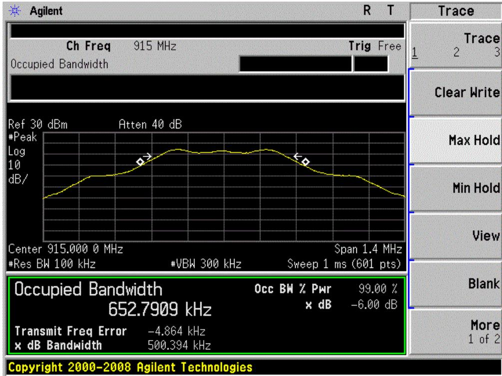
6dB Bandwidth plot on channel 02
