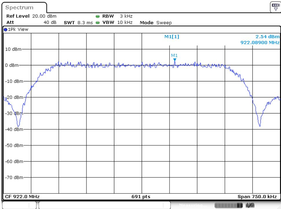
Power spectral density plot on channel 03
