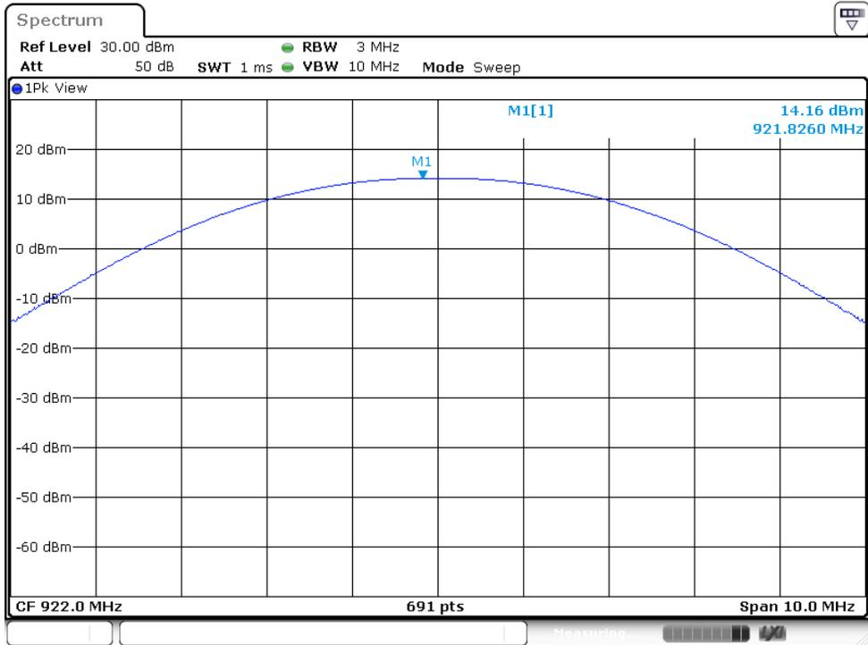
Peak output Power plot on channel 03
