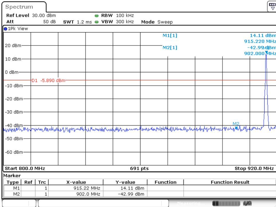
GFSK mode: Band Edge-High Channel
