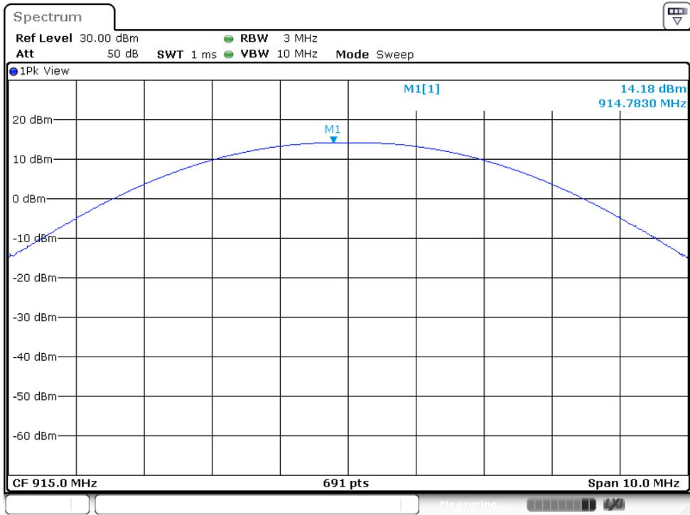
Peak output Power plot on channel 02
