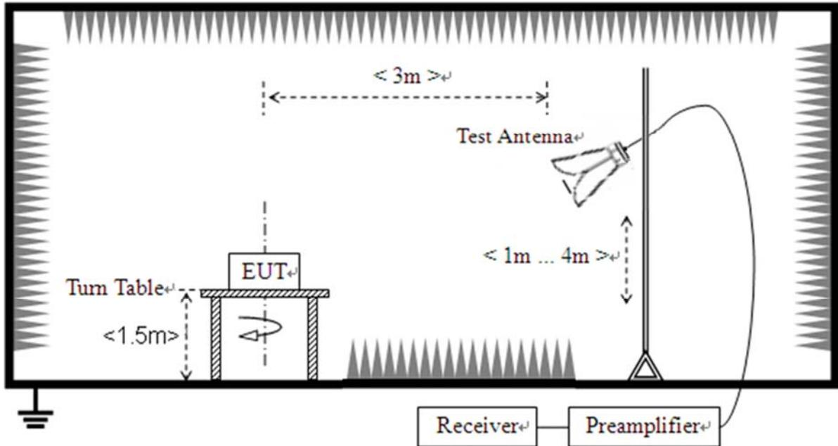
The EUT is placed on a non-conducting table 80 cm above the ground plane for measurement below 1GHz; 1.5 m above the ground plane for measurement above 1GHz. The antenna to EUT distance is 3 meters. The EUT is configured in accordance with ANSI C63.10. The EUT is set to transmit in a continuous mode.
