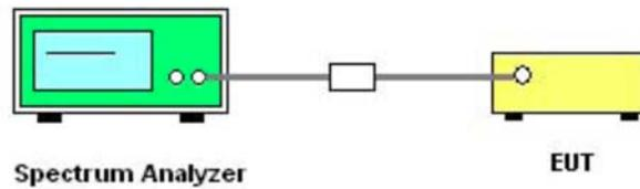
The EUT is coupled to the Spectrum Analyzer; the RF load attached to the EUT antenna terminal is 50Ohm; the path loss as the factor is calibrated to correct the reading.
