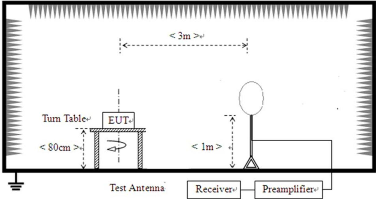
2) For radiated emissions from 30MHz to 1GHz
