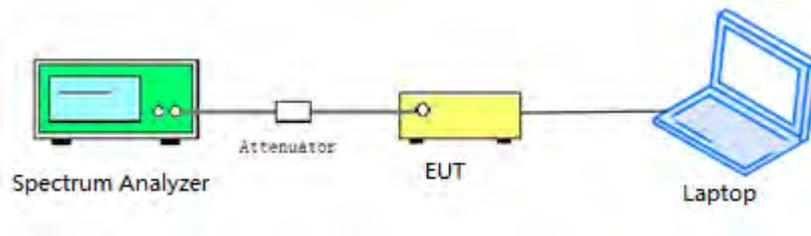
The EUT is coupled to the Spectrum Analyzer; the RF load attached to the EUT antenna terminal is 50Ohm; the path loss as the factor is calibrated to correct the reading.
