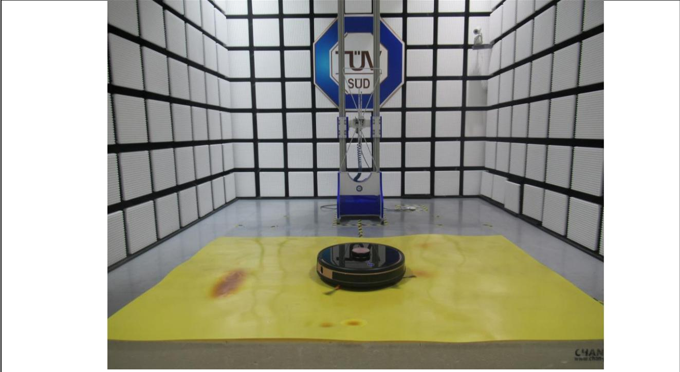
Test setup of: Spurious Radiated Emissions (1-18 GHz)
