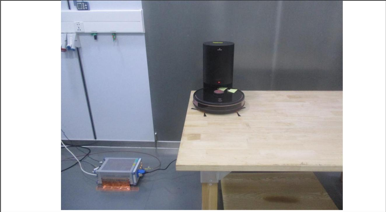
Test setup of: Spurious Radiated Emissions (Below 1 GHz)
