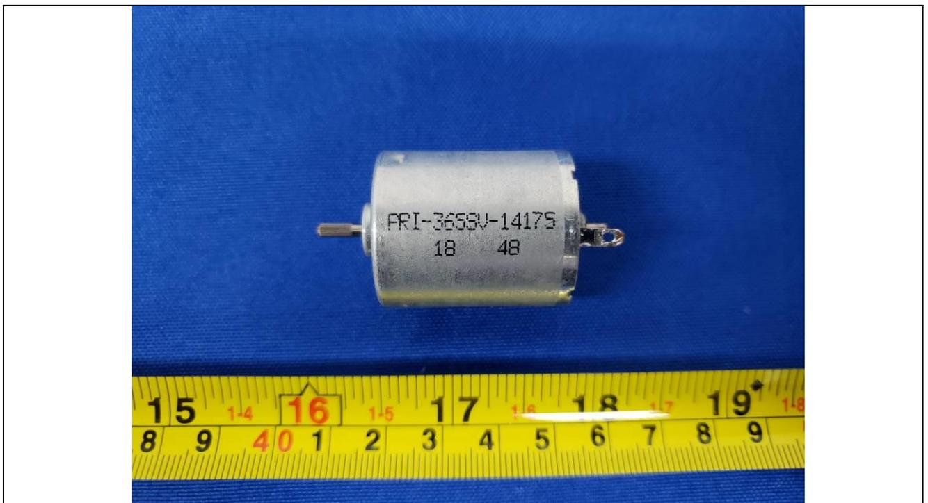
Details of: Rotary brush motor (for PR-500EV-10470-31.5CB)
