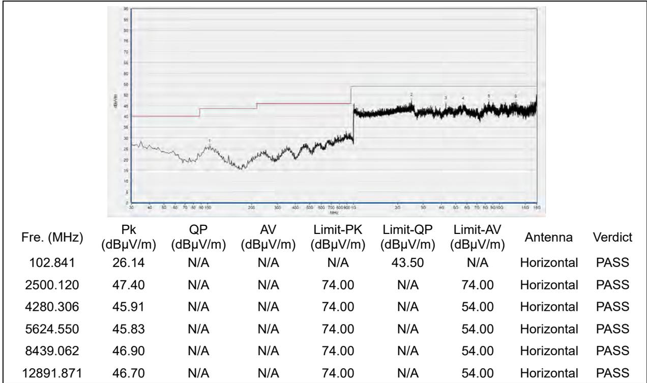
(30MHz to 25GHz, Antenna Horizontal, GFSK, channel 39)
