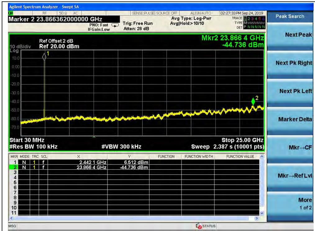
(Channel = 39, 30MHz to 25GHz, GFSK Mode)
