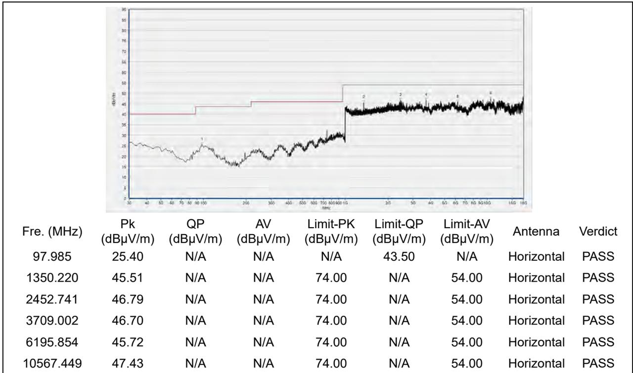
(30MHz to 25GHz, Antenna Horizontal, GFSK, channel 0)
