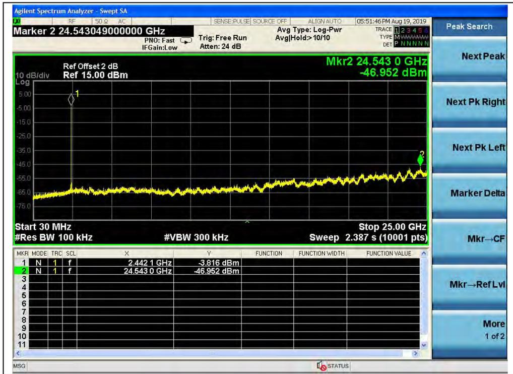
(Channel = 39, 30MHz to 25GHz,  $\pi/4$ -DQPSK)
