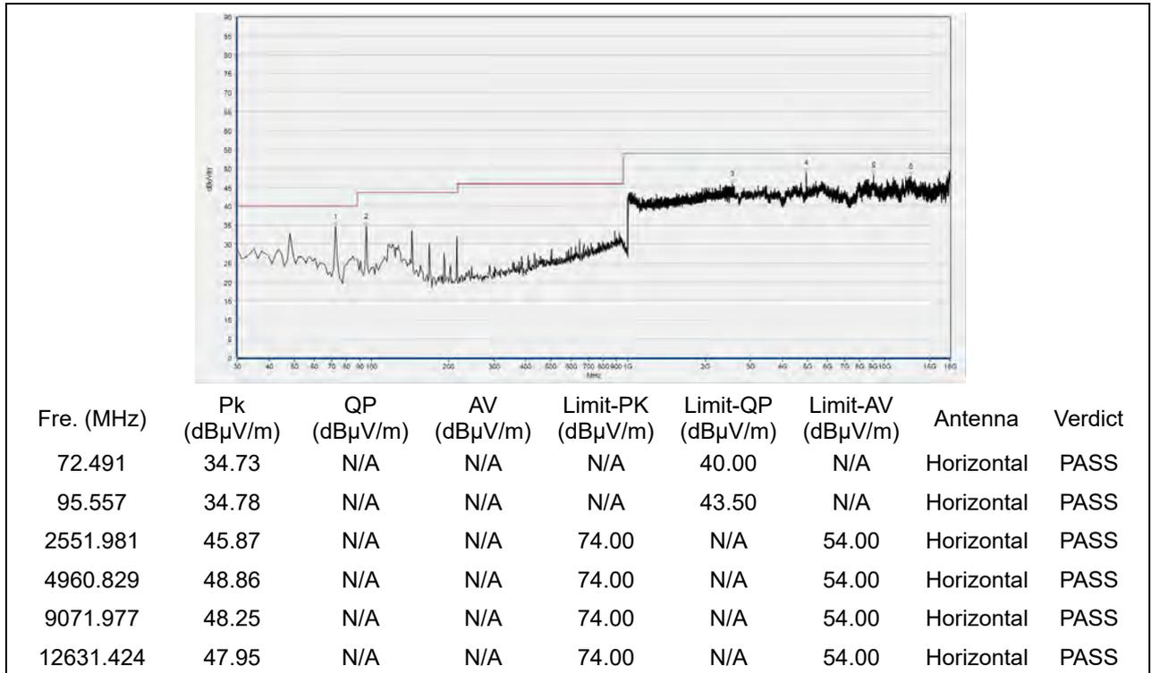
(30MHz to 25GHz, Antenna Horizontal, GFSK, channel 78)
