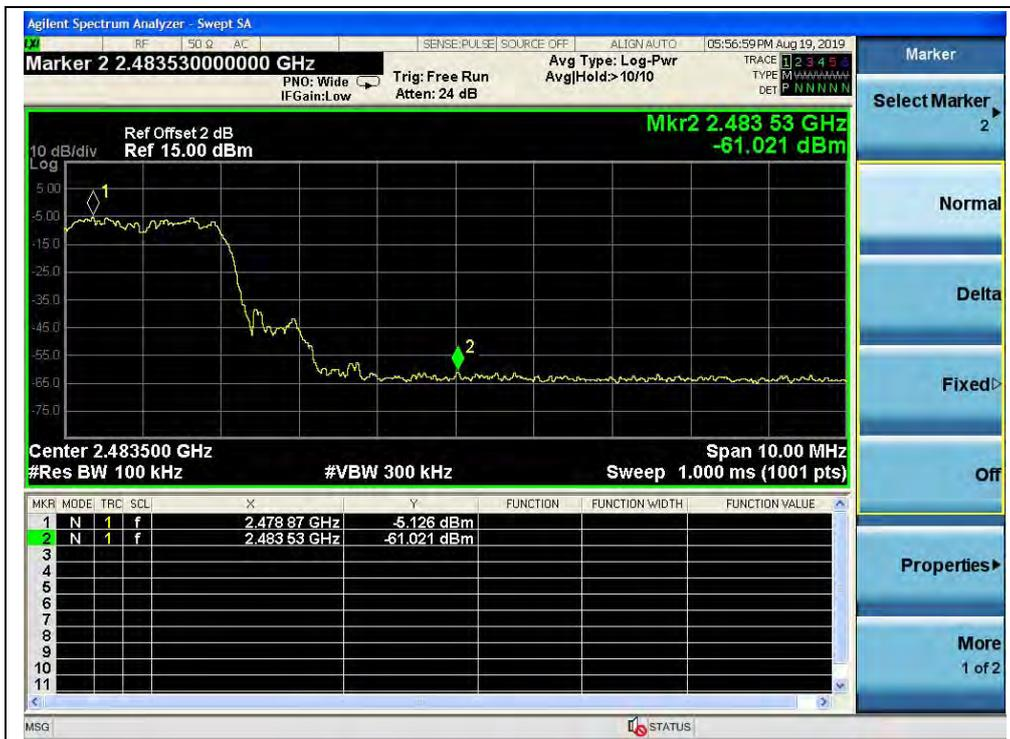
(Channel = 78, Band edge with hopping on, 8-DPSK)
