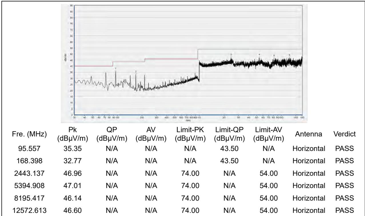
(30MHz to 25GHz, Antenna Horizontal, 8-DPSK, channel 0)
