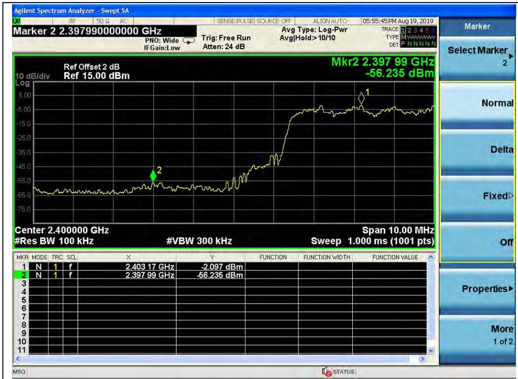
(Channel = 0, Band edge with hopping on, 8-DPSK)
