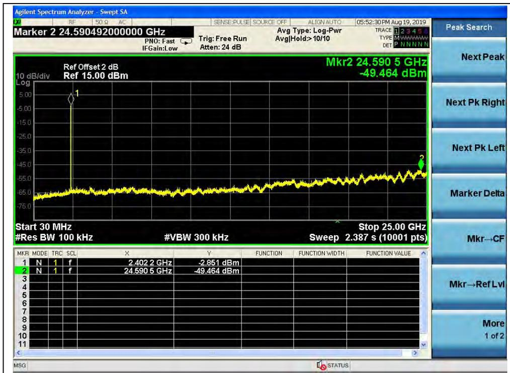
(Channel = 0, 30MHz to 25GHz,  $\pi/4$ -DQPSK)
