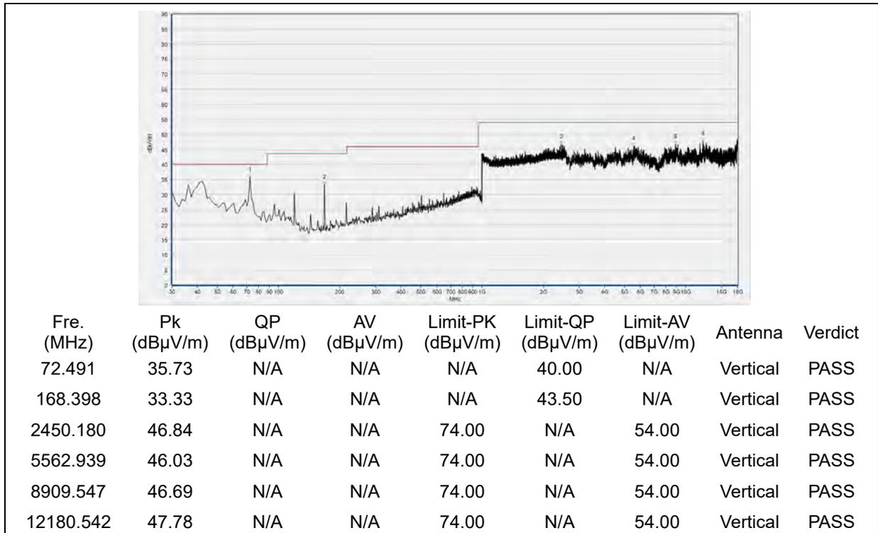
(30MHz to 25GHz, Antenna Vertical, GFSK, channel 39)
