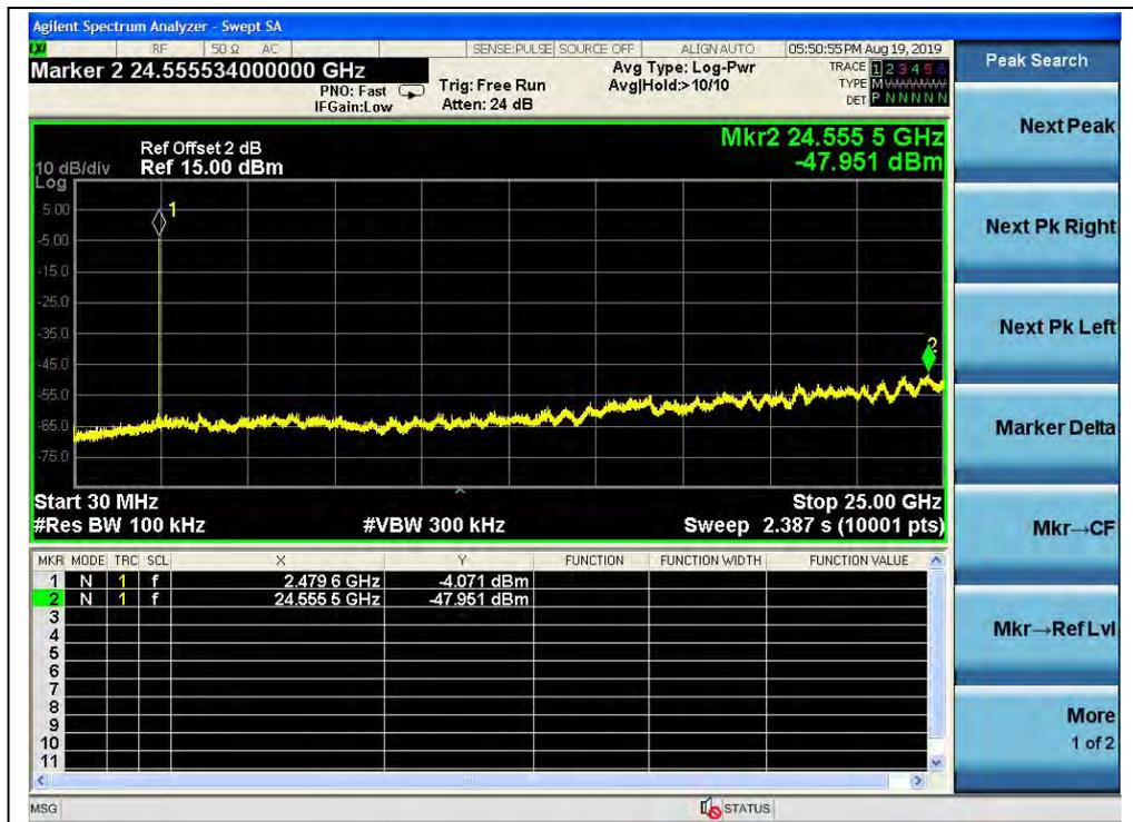
(Channel = 78, 30MHz to 25GHz,  $\pi/4$ -DQPSK)
