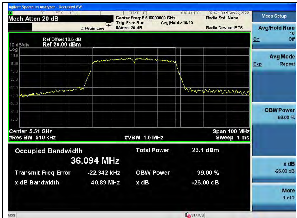
(Channel 102, 5510MHz, 802.11ac (VHT40))
