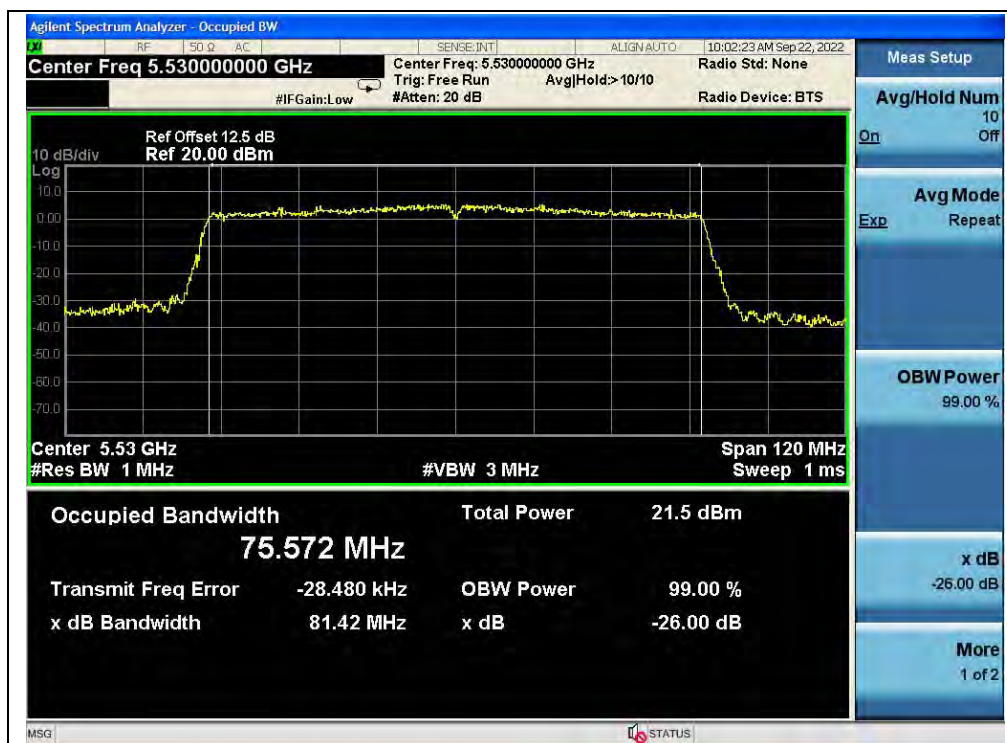
(Channel 106, 5530MHz, 802.11ac (VHT80))
