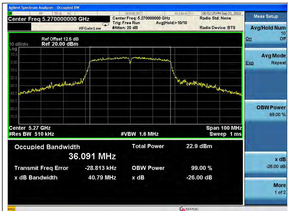
(Channel 54, 5270MHz, 802.11ac (VHT40))
