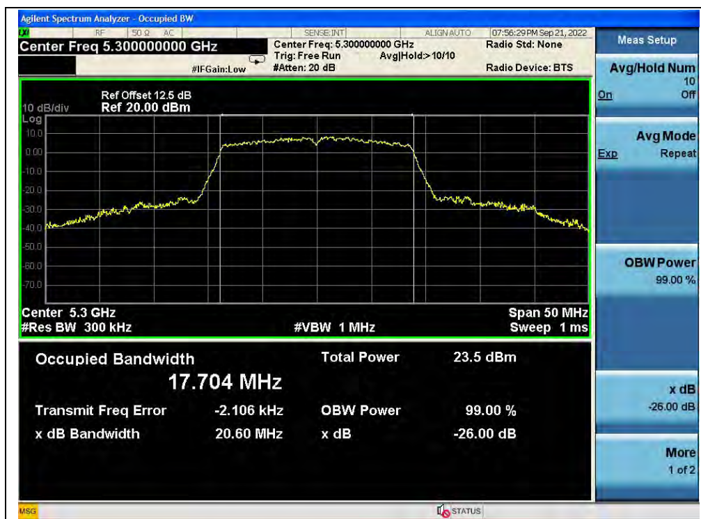
(Channel 60, 5300MHz, 802.11ac (VHT20))
