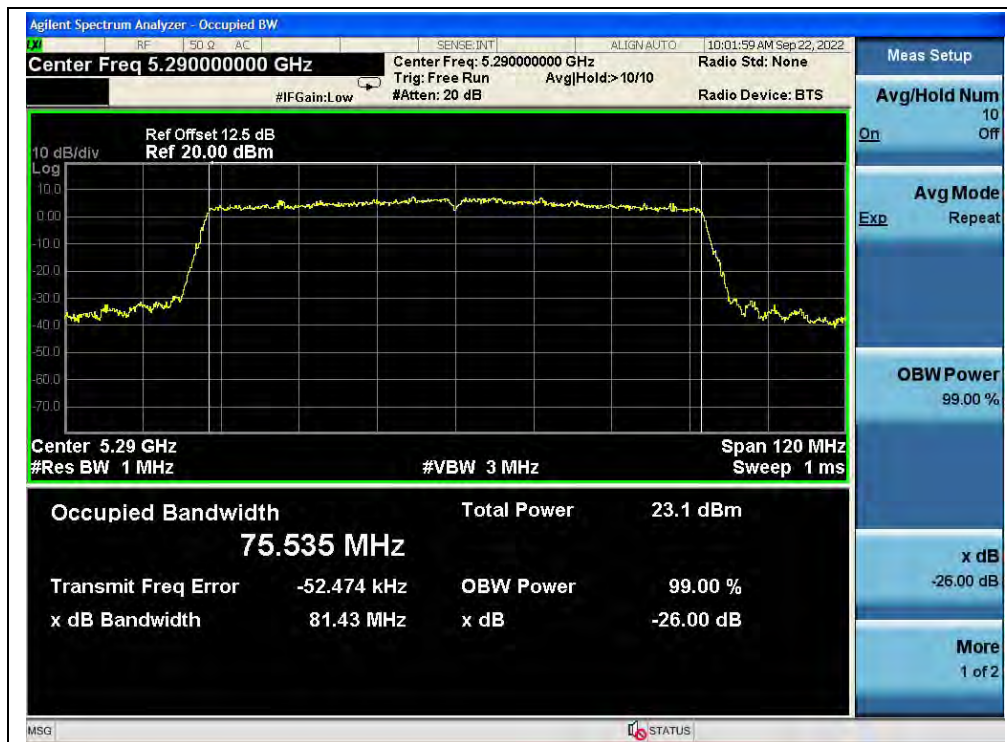
(Channel 58, 5290MHz, 802.11ac (VHT80))
