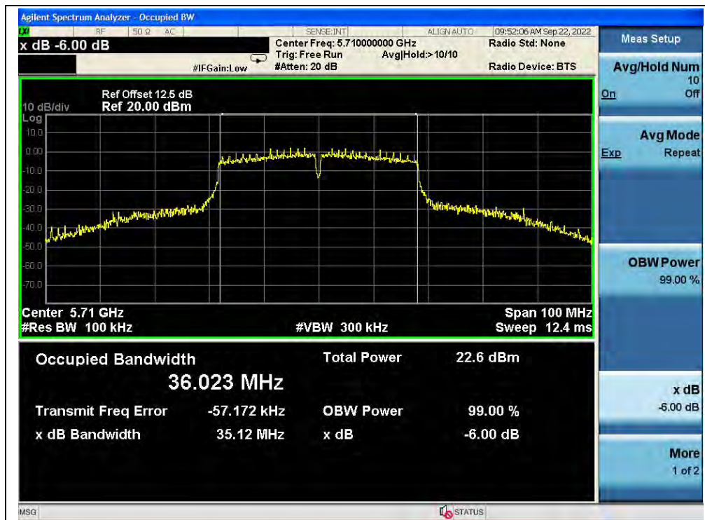
(Channel 142, 5710MHz, 802.11ac (VHT40))
