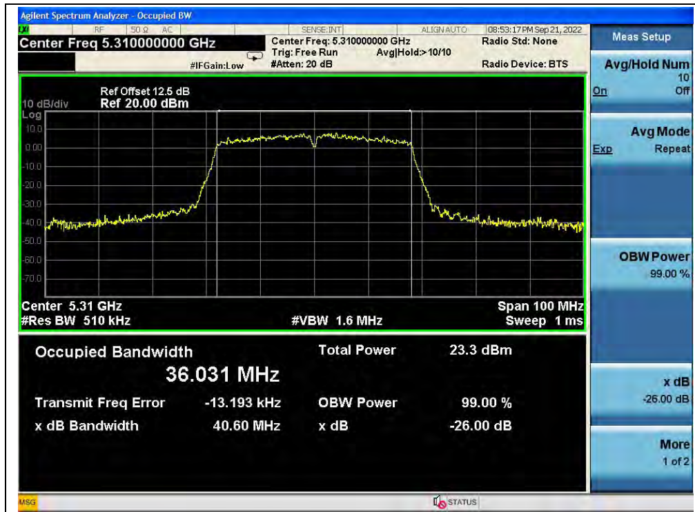
(Channel 62, 5310MHz, 802.11ac (VHT40))
