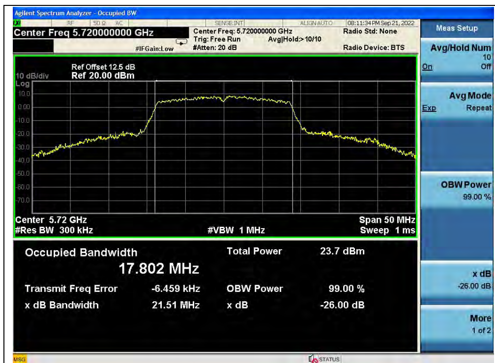
(Channel 144, 5720MHz, 802.11ac (VHT20))
