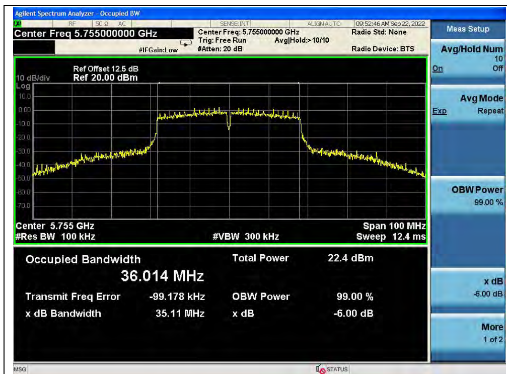
(Channel 151, 5755MHz, 802.11ac (VHT40))
