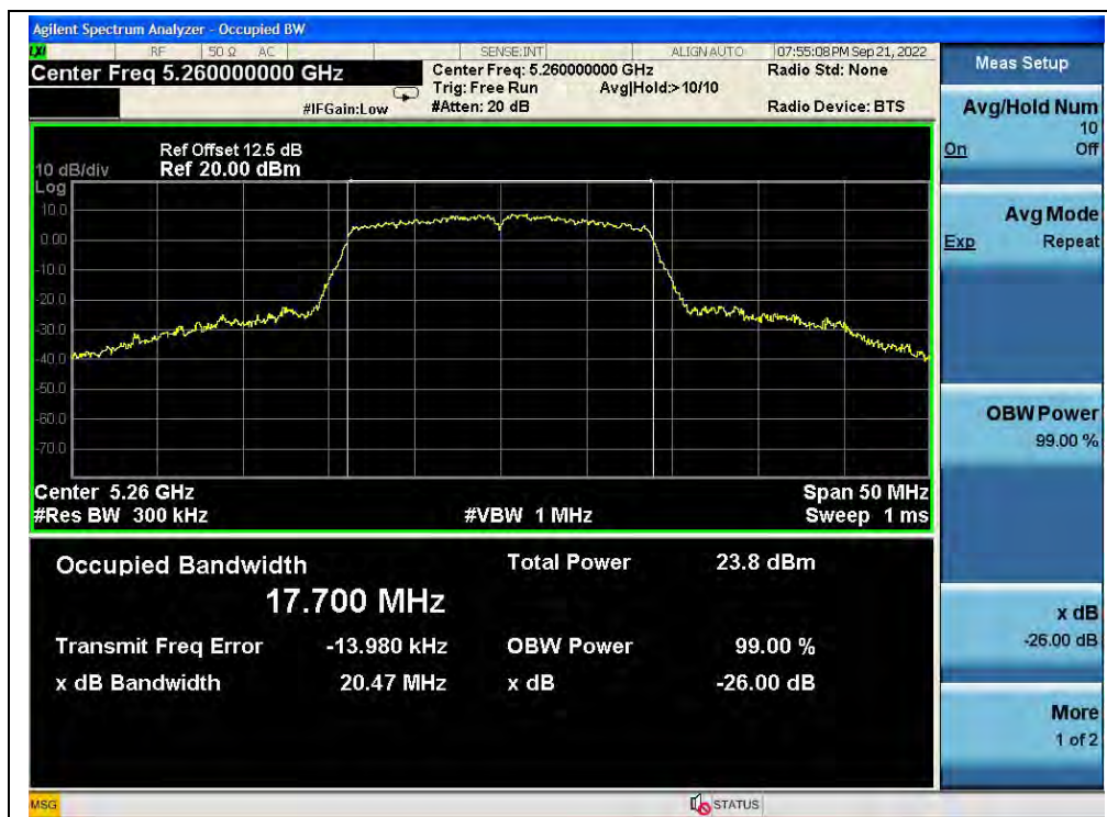
(Channel 52, 5260MHz, 802.11ac (VHT20))
