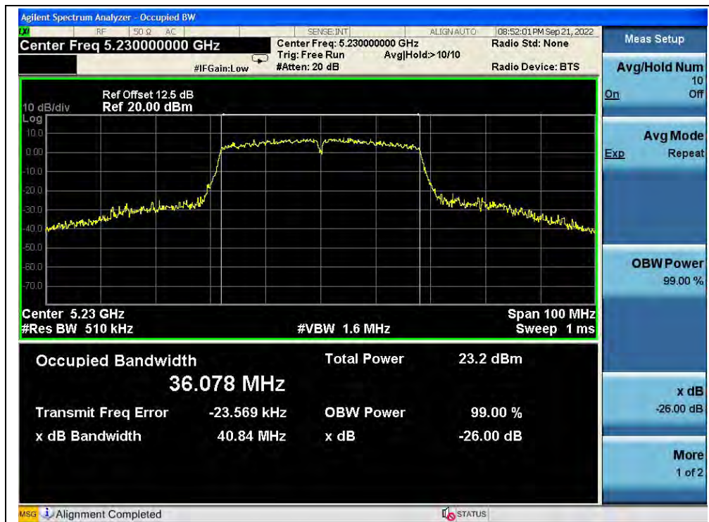
(Channel 46, 5230MHz, 802.11ac (VHT40))
