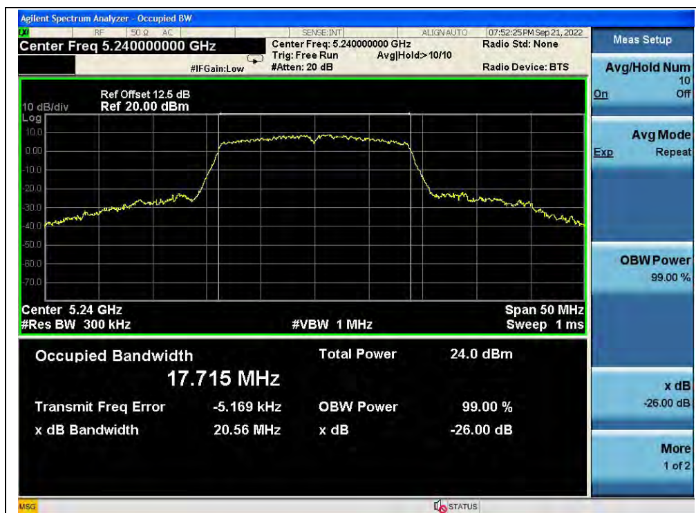
(Channel 48, 5240MHz, 802.11ac (VHT20))
