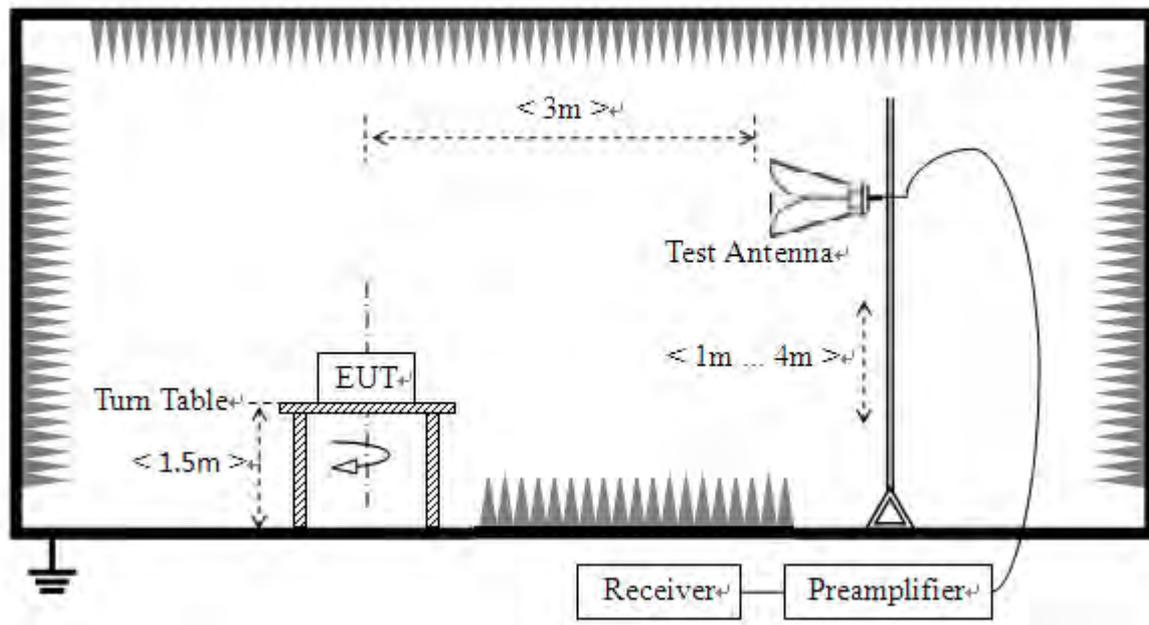
The EUT is located in a 3m Semi-Anechoic Chamber; the antenna factors, cable loss and so on of the site as factors are calculated to correct the reading. During the measurement, the Bluetooth Module of the EUT is activated and controlled by the Bluetooth Service Supplier (SS) via a Common Antenna, and is set to operate under non hopping-on test mode transmitting 339 bytes DH5, 679 bytes 2DH5 and 1021 bytes 3DH5 packages at maximum power.
