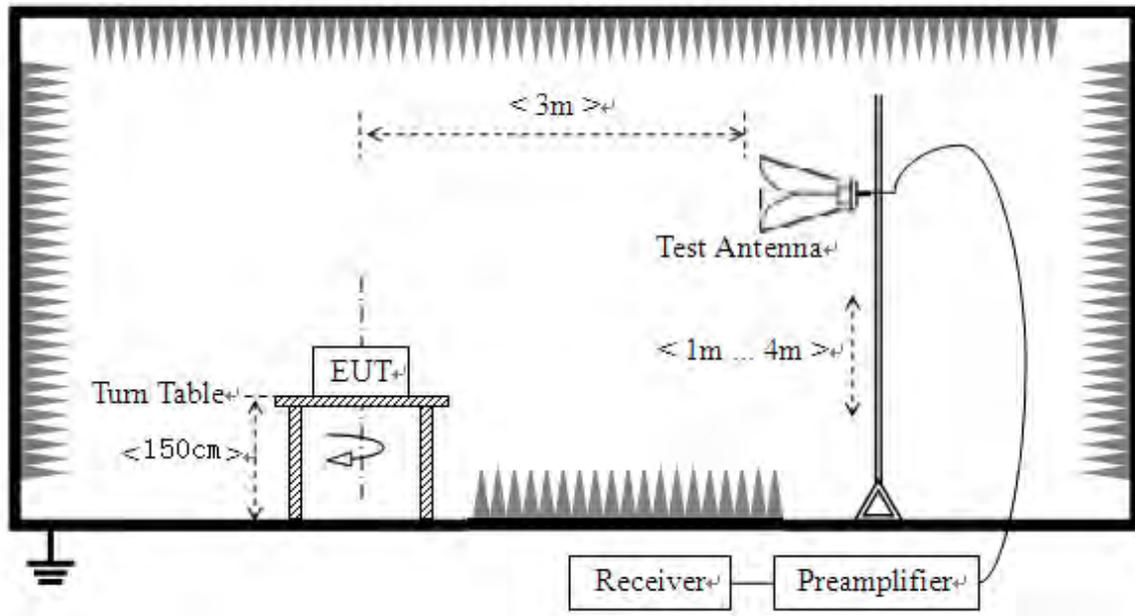
The RF absorbing material used on the reference ground plane and on the turntable have a maximum height (thickness) of 30 cm (12 in) and have a minimum-rated attenuation of 20 dB at all frequencies from 1 GHz to 18 GHz. Test site have a minimum area of the ground plane covered with RF absorbing material as specified in Figure 6 of ANSI C63.4: 2014.
