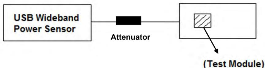
The EUT (Equipment under the test) which is coupled to the USB Wideband Power Sensor; the RF load attached to the EUT antenna terminal is 50Ohm; the path loss as the factor is calibrated to correct the reading, all test result in USB Wideband Power Sensor.
