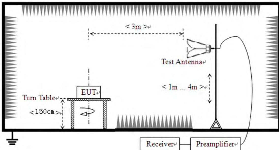
The Module is located in a 3m Semi-Anechoic Chamber; the antenna factors, cable loss and so on of the site as factors are calculated to correct the reading.
