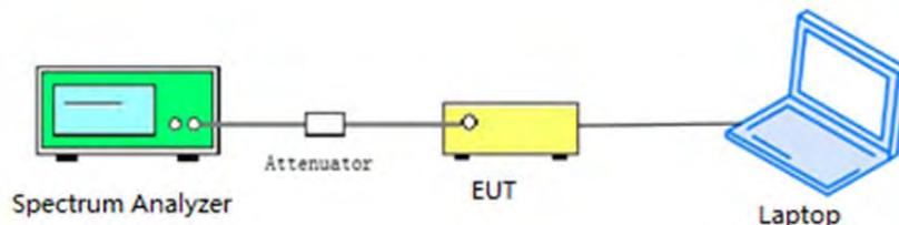
The EUT is coupled to the Spectrum Analyzer; the RF load attached to the EUT antenna terminal is 50 Ohm; the path loss as the factor is calibrated to correct the reading.
