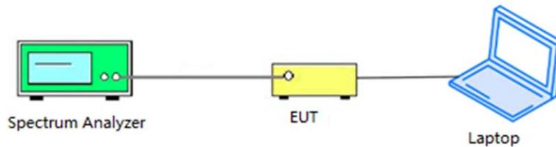
The EUT (Equipment under the test) is coupled to the Spectrum analyzer; the RF load attached to the EUT antenna terminal is 50Ohm; the path loss as the factor is calibrated to correct the reading, all test result in Spectrum analyzer.
