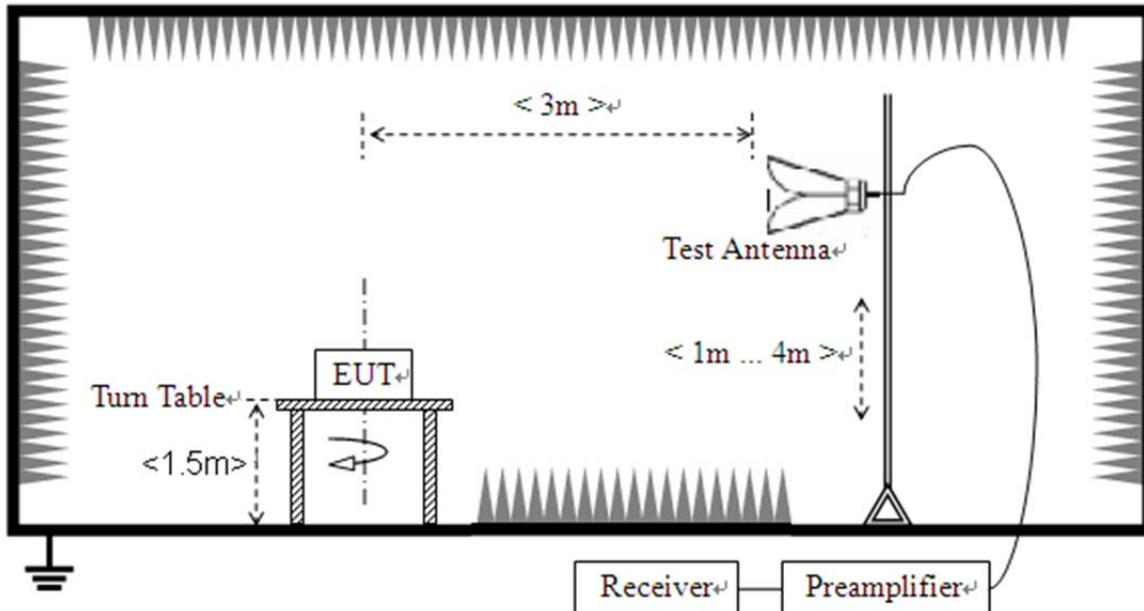
The RF absorbing material used on the reference ground plane and on the turntable have a maximum height (thickness) of 30 cm (12 in) and have a minimum-rated attenuation of 20 dB at all frequencies from 1 GHz to 18 GHz. Test site have a minimum area of the ground plane covered with RF absorbing material as specified in Figure 6 of ANSI C63.4: 2014.
