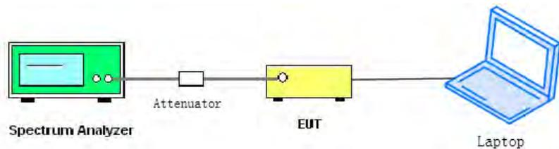
The EUT is coupled to the Spectrum Analyzer; the RF load attached to the EUT antenna terminal is 50Ohm; the path loss as the factor is calibrated to correct the reading.
