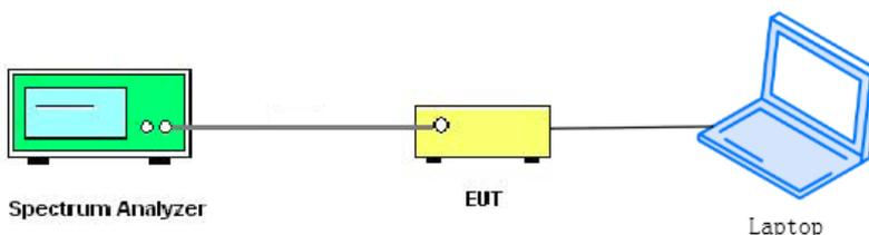
The EUT (Equipment under the test) is coupled to the Spectrum analyzer; the RF load attached to the EUT antenna terminal is 50Ohm; the path loss as the factor is calibrated to correct the reading, all test result in Spectrum analyzer.
