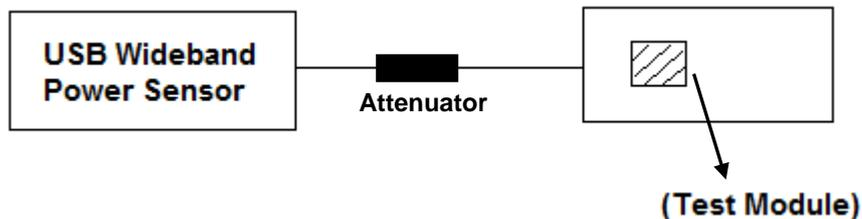
The EUT (Equipment under the test) which is coupled to the USB Wideband Power Sensor; the RF load attached to the EUT antenna terminal is 50Ohm; the path loss as the factor is calibrated to correct the reading.
