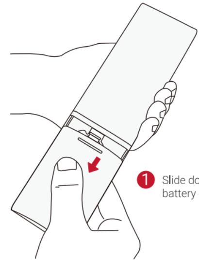
1 Slide down to open the battery compartment.
