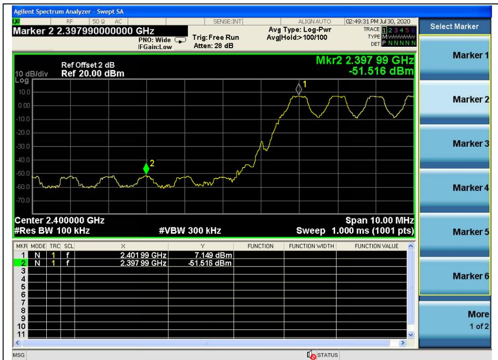
(Band edge with hopping on, Channel 0, GFSK)
