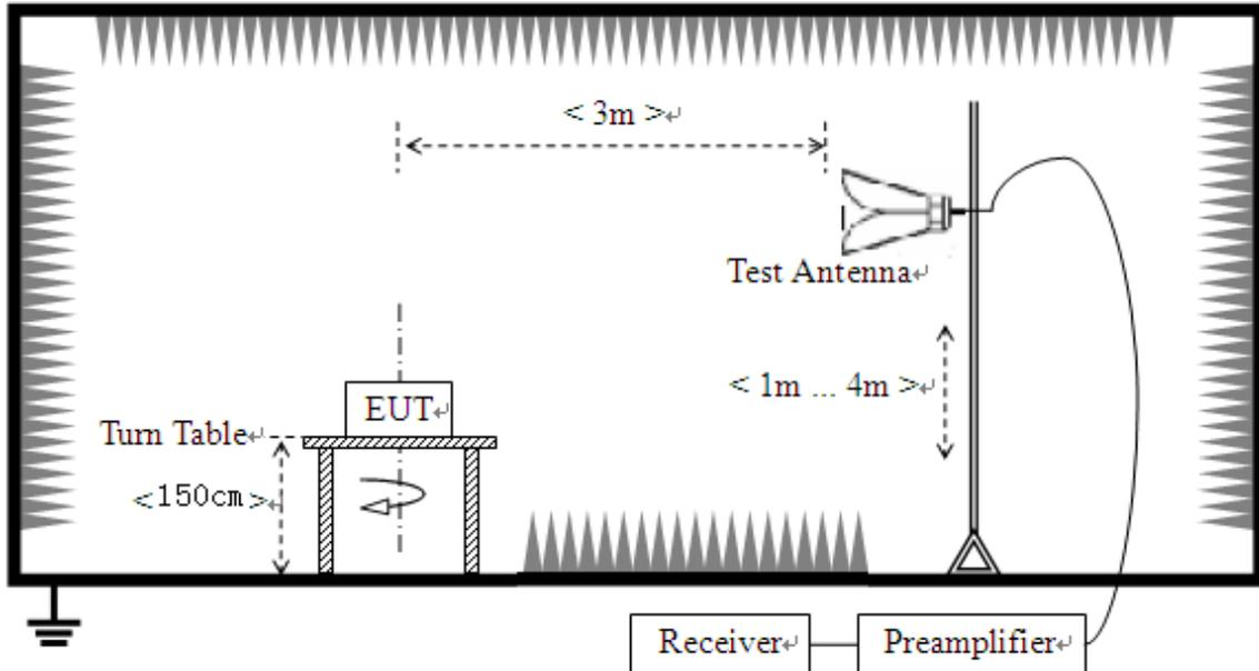
The RF absorbing material used on the reference ground plane and on the turntable have a maximum height (thickness) of 30 cm (12 in) and have a minimum-rated attenuation of 20 dB at all frequencies from 1 GHz to 18 GHz.
