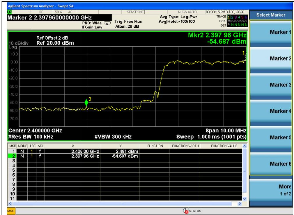
(Band edge with hopping on, Channel 0, 8-DPSK)
