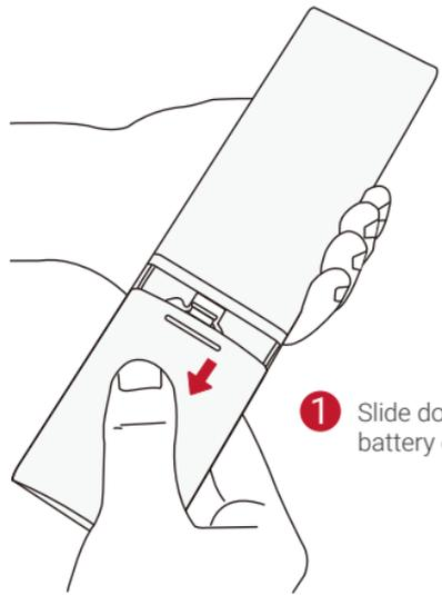
1 Slide down to open the battery compartment.
