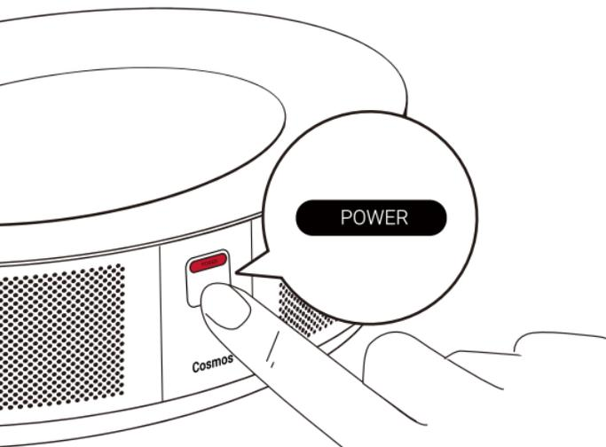
Press **POWER** to power on. Press and hold **POWER**. A menu pops up. Select Power Off to turn off the projector.
