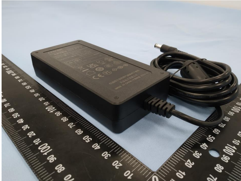
Photograph 13: Support Units (Switching Power Supply)
