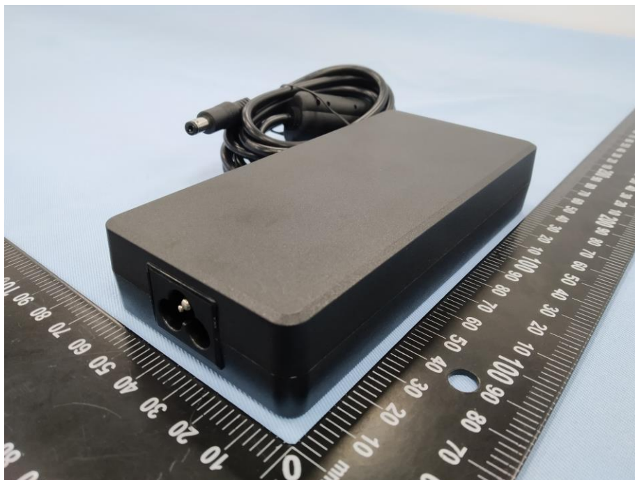
Photograph 12: Support Units (Switching Power Supply)
