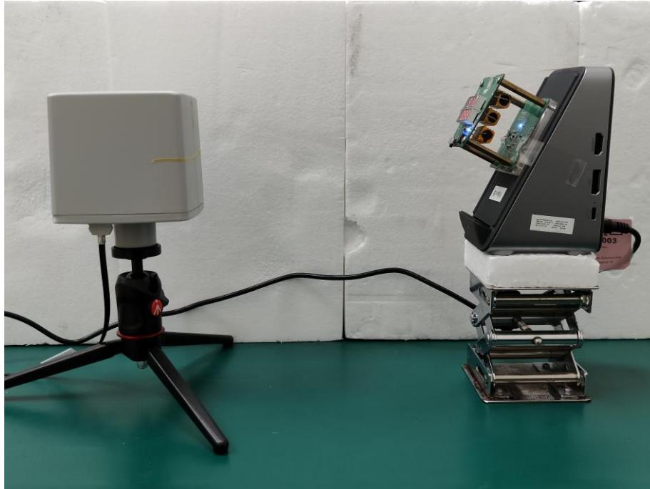
Photograph 6: Set-up for H-field strength (Front View)
