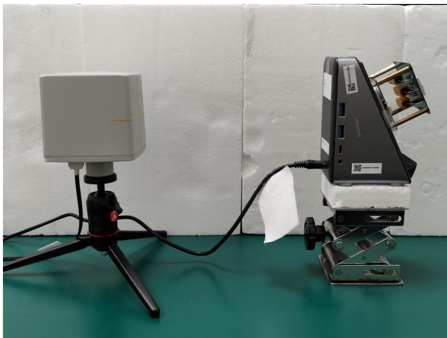
Photograph 7: Set-up for H-field strength (Back View)
