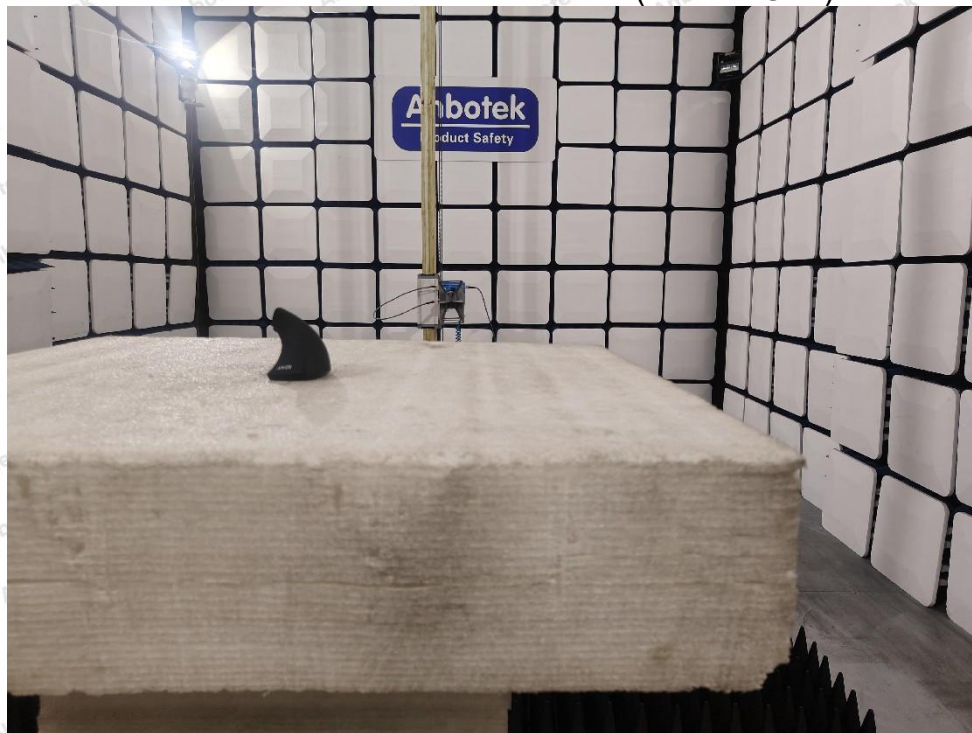
Photo of Radiation Emission Test (above 1GHz)
