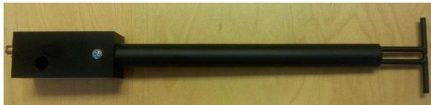
**Figure 1 – MVG COMOSAR Validation Dipole**
